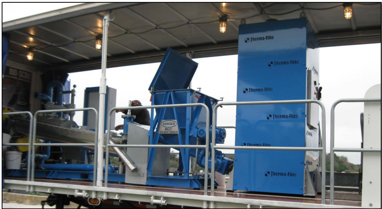
Trailer-mounted Indirect Drying System with Dryer, Wet Feed (Cake) Hopper, and Heater Unit
